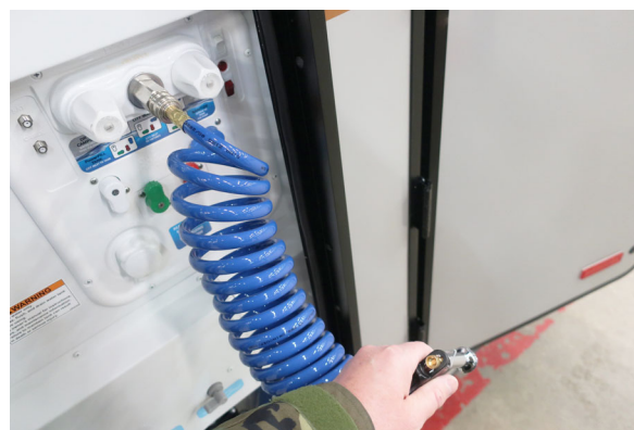
Exterior Shower/Wash Station (located in the drivers side service center, shown with shower hose hooked up. -Typical View)
