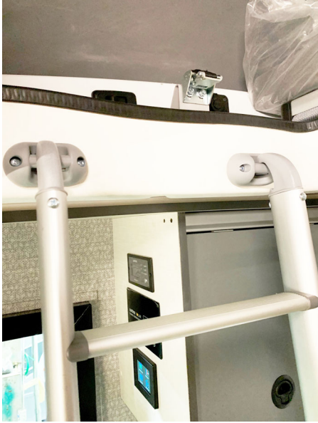
Attach the ladder to the attachment points located on the passenger side. The ladder hooks in from the top. -Typical View
