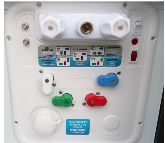
Water Center Panel shown in the “blow out” configuration. -Typical View
