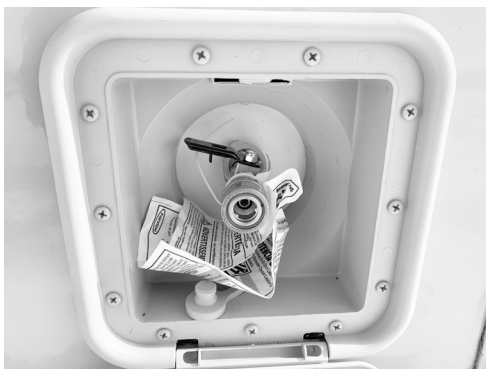
LP Quick Connect Port (shown open). Located on the passenger side. -Typical View
