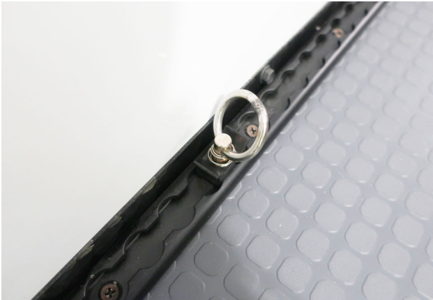
View of one of the retention hooks. Pull out on the ring while holding down the base to unlock and move to another location on the track. -Typical View
