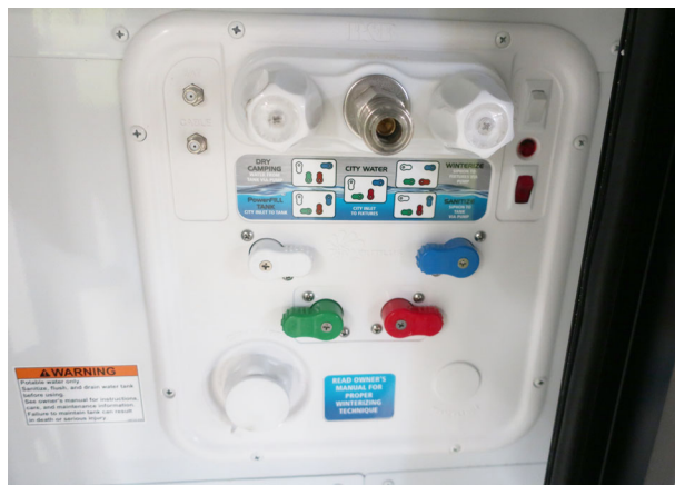
Water Center Panel in “Winterize” configuration (Panel located inside the service center on the drivers side).
