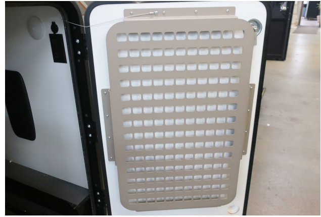
MOLLE Panel on the Passenger side Gear Garage access door. -Typical View
