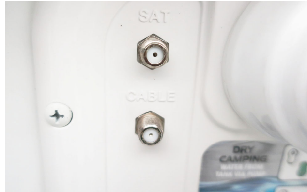
Satellite Dish and Cable TV Connections (Located on the Water Center Panel) -Typical View
