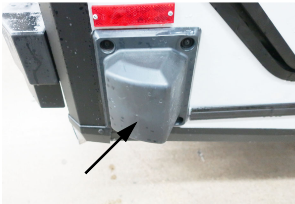
Passenger side blind spot sensor location. Do not paint or cover this block. -Typical View
