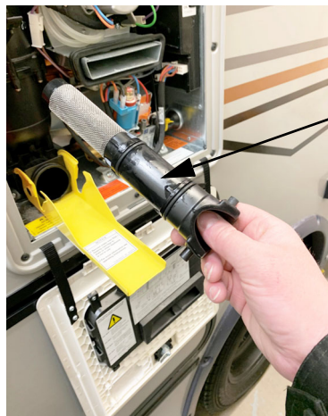
Water inlet filter pulled out and removed. -Typical View
