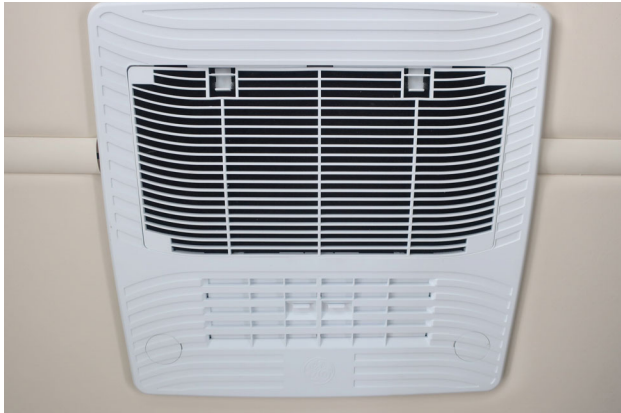
Air conditioner vent located at the rear of the motorhome. -Typical View
