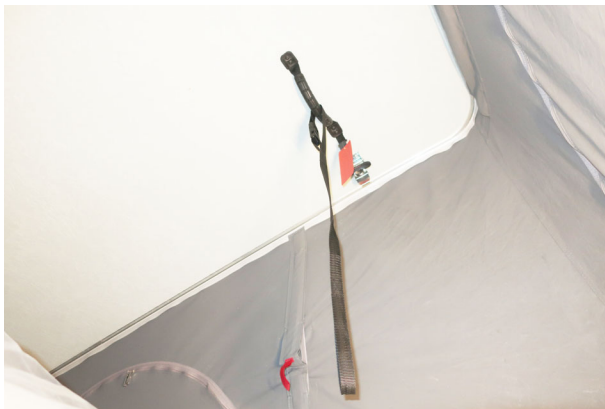
Reverse the steps to collapse the Pop-Top into the travel position. Use the straps that are attached to the handles to assist pulling the Pop-Top down. The red tab handles located on the sides are designed to pull the material inward, to ensure that the Pop-Top does not close down and pinch itself. -Typical View
